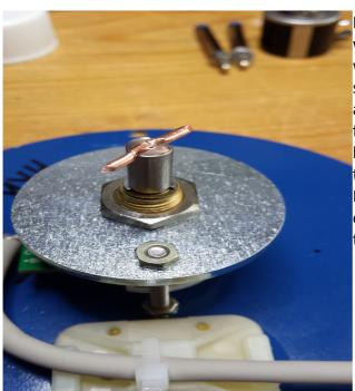
Now for the guiding pin. I cut some 15 mm copper wire (diameter 1.5 mm), salvaged from installation wire. With a small hammer, or if you are very strong with tweezers, squeeze the central part so as to fit the slit in the sensor. Try not to engage force on the sensor, just on its shaft. So do not hammer the pin in! If it fits snugly then apply a tiny drop of glue. Picture left.
