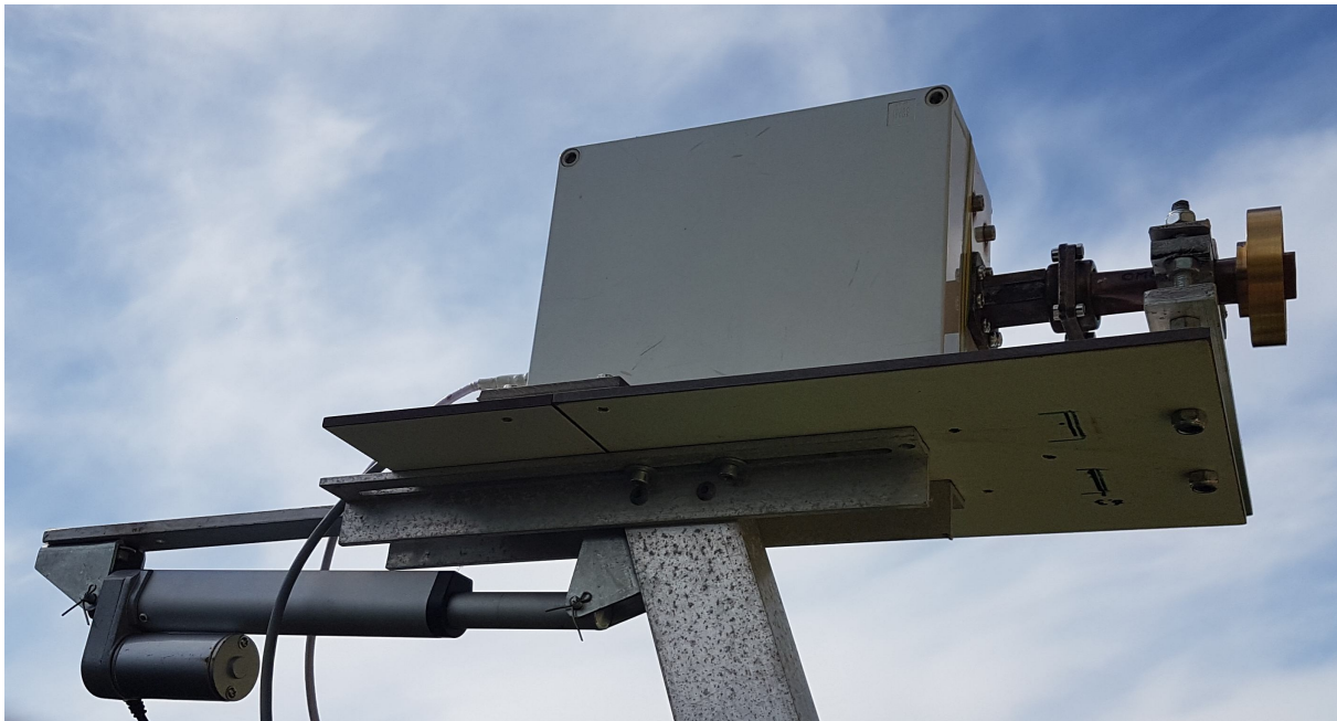
Remote controlled actuator for optimal focus positioning.
